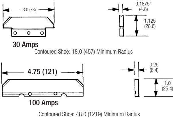
Standard shoe material is copper graphite. The optional cast iron shoe is to be used temporarily to clean the bar. "Insuloy" has self-cleaning properties, but will cause more wear on the bar versus copper graphite.
