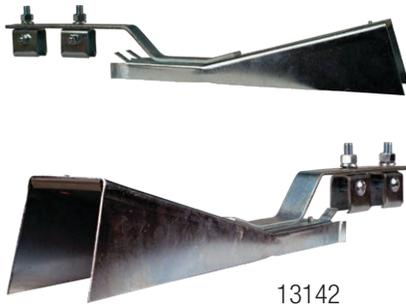
The Pick-up Guide allows the collector to leave the conductor and re-track upon return. Requires use of "Self-Centering" J-Head Collectors, see pages 23-24. Contact factory for selection.
