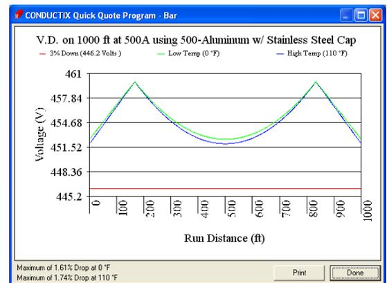
**Figure 4:** Two power feeds optimally located. The voltage drop remains under 3%, without the need to increase conductor capacity. A load positioned between the two feed points is supplied by both power feeds.
