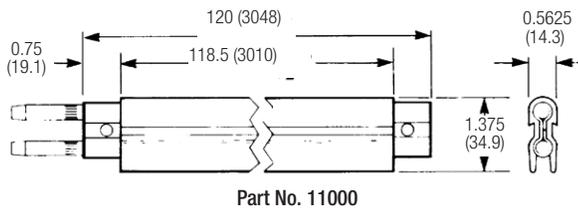
Roll formed of 1/16" (1.59 mm) material except laminates which are 1/32" (0.79 mm) copper, steel, or stainless steel, and the 90 A galvanized bar. The cross-section area is 188 mcm (95 mm<sup>2</sup>). The equivalent rectangle for all conductors is 1" x 1/4" (25.4 x 6.3 mm). Supports are required every 3 feet (0.91 M) for curves, 3 feet 4 inches (1.01 M) for lateral mount, and 5 feet (1.52 M) standard.
