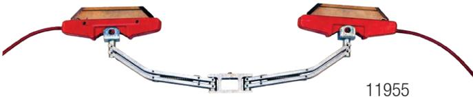
Continuous systems that require 80A capacity. Operates through curves to minimum radii of 24.0 (610). Has tandem collectors.
