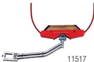
For conveyor, monorail systems, and crane bridges. Operates through curves at a minimum radii of 9.0 (228). Includes an additional pigtail for extra current capacity.
