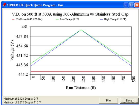
**Figure 1 – Center Feed Example:** Voltage drop along a 500 foot (152.4 meters) long runway with one crane drawing 500 amps at 460 volts on a 500 amp rated bar. The green line shows the voltage drop along the run at 0° F. The blue line shows the voltage drop at 110° F. The red line indicates the 3% maximum voltage drop. The voltage drop increases linearly as you move away from the center feed point.
