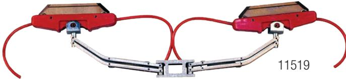
For systems that require 160A capacity. Operates through curves to minimum radii of 24.0 (610). Has tandem collectors and additional pigtails for the added current capacity.
